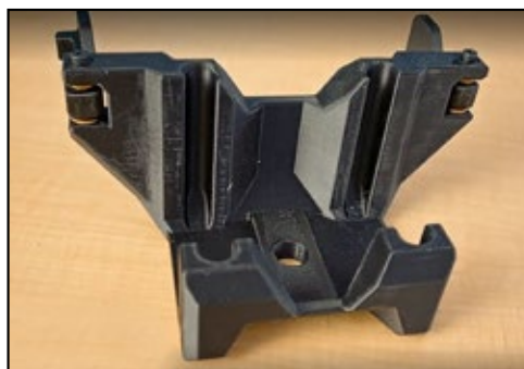
In contrast, the 3D printed fixture on the right serves the same purpose but is made up of fewer parts and can be printed in a single print operation.
