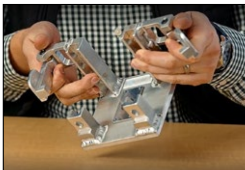
The assembly fixture on the left is made up of multiple parts that are welded and pinned together.
